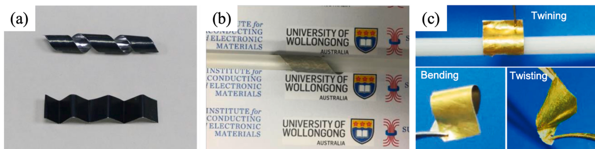
Fig. 17. a) MXene-coated zinc foil at twisting and bending tests [54]. b) ZnS-coated zinc foil at twisting test [26]. c) F-COF-coated zinc foil at twining, bending, and twisting tests [91].
